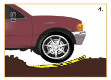
In the event there is difficulty in gaining grip onto the recovery track, reverse the vehicle onto the already compressed ground, then move forward with sufficient momentum to mount the recovery track.
