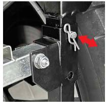
**4.** Use the adjustable rubber bumpers to protect your wheels and ensure the step is sturdy and level.
