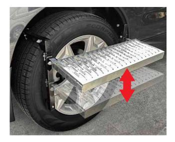
**3A.** Insert the supplied bolt into position and secure with the R-Clip on both sides of the wheel step.
