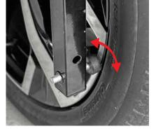
NOTE In order to prevent the screws from loosening when in use, the screws must be screwed inside as far as possible, preferably parallel to the other hole of the square tube.
