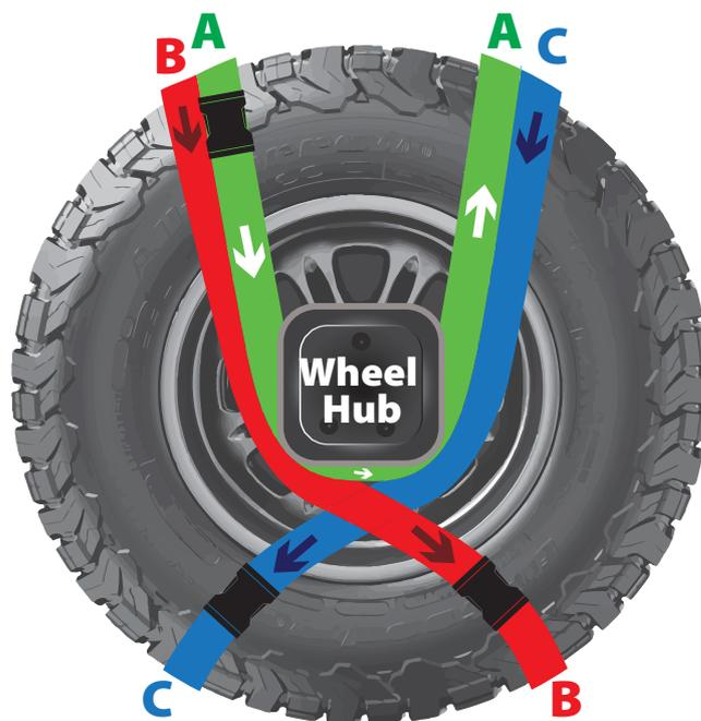
**Step 4.** Feed the left (B) and right (C) hand straps over and behind the tyre in a criss cross motion, attaching the quick connect buckle to the opposite side of the tyre.
